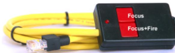
To remind yourself of the button functions, press the buttons whilst not connected to the camera. The red LED indicates that "fire" was pressed.
