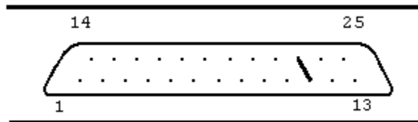
Link for Watchdog test LED connector, DB-25F (holes) seen from the outside of the box.
